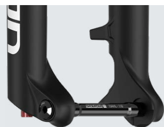
15AHL (TOOL TYPE) Ø15mm, O.L.D.: 110mm Weight: 42g
