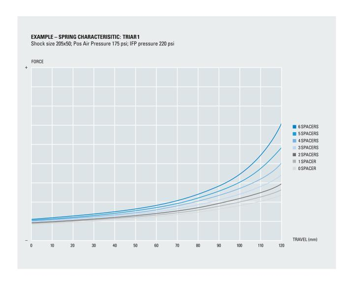
Adjust your spring curve by using different amount of plastic volume spacers part FAA123.
