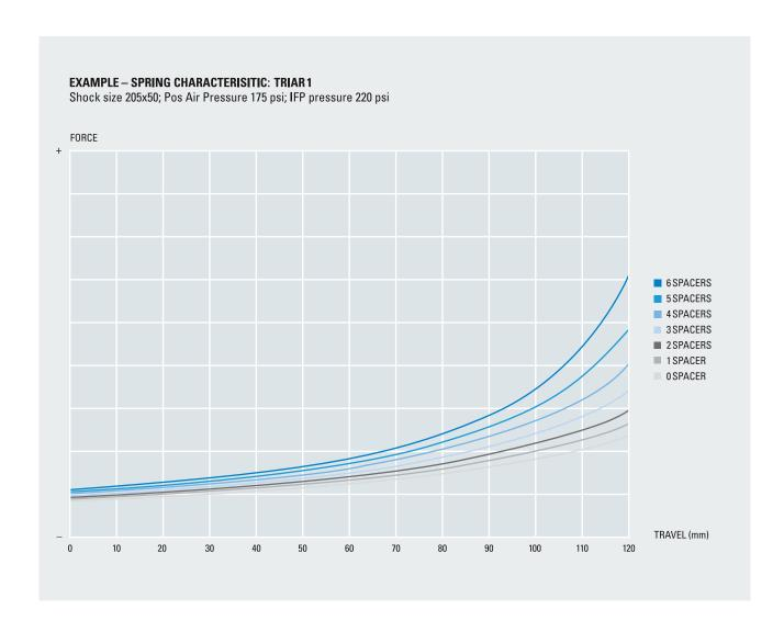
Adjust your spring curve by using different amount of plastic volume spacers part RAA123.
