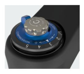
To open the low speed compression: Turn counter clockwise towards the (-). Result: You get a supple feel with sensitivity on small bumps. To close the low speed compression: Turn clockwise towards the (+). Result: The more you close, the more support you get. Compression feeling is firmest.
