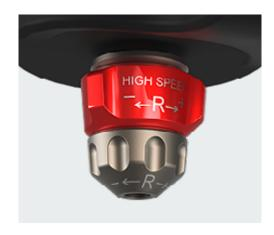
To open the low speed rebound: Turn the knob clockwise toward the (-) to open the low speed rebound. Result: The global rebound speed is faster.
