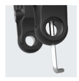
To open the rebound: Use a 3mm Allen key that you insert in the center of the screw. Turn counter clockwise toward the (-) Result: The global rebound speed is faster.
