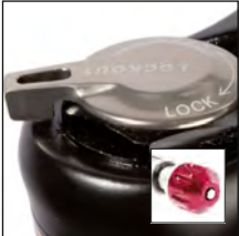
LO-R Speed Lock out Rebound adjust
