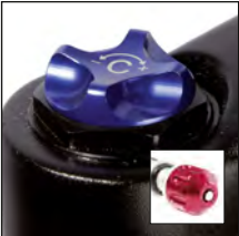
RC Rebound adjust Low speed Compression adjust
