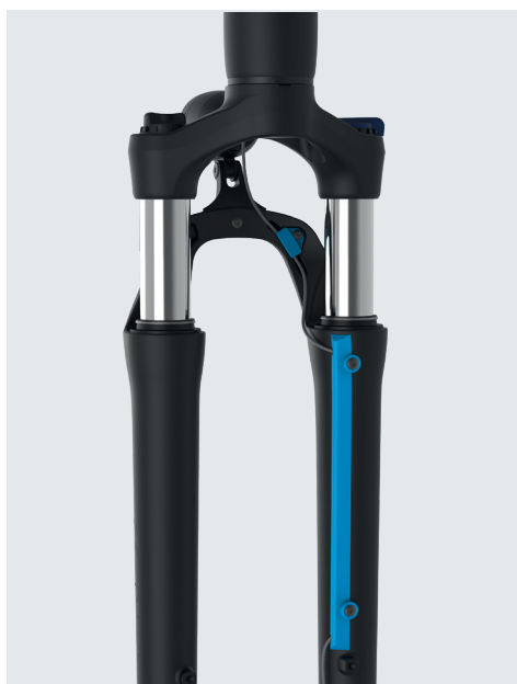
HUB DYNAMO CABLE GUIDE w/screws *Option
