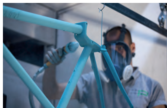
TOP We love welding. We love handmade bikes. LEFT Before the frames gets the powder coating the surface needs to be treated by sandblasting and a lavation.
