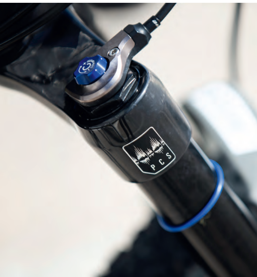
NLO Hydraulic Lockout with fixed rebound damping.
