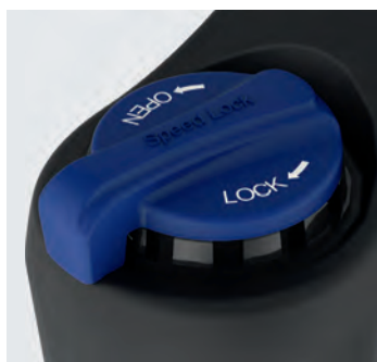
NLO Hydraulic Lockout with fixed rebound damping.
