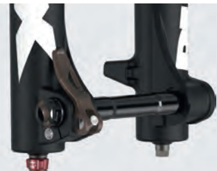
QR (TOOL FREE) Ø20mm, O.L.D.: 110mm Weight: 120g
