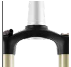
AC4C: Accurad Forging Technology (geschmiedete Krone)
