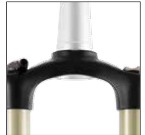
AC4C: Accurad Forging Technology (solid crowns)
