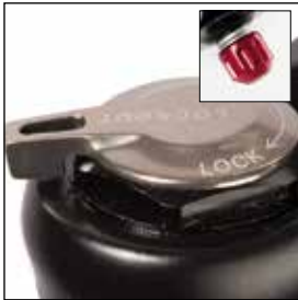
LO R: Rebound adjust + speed lock out
