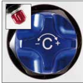
RC: Low Speed Compression
