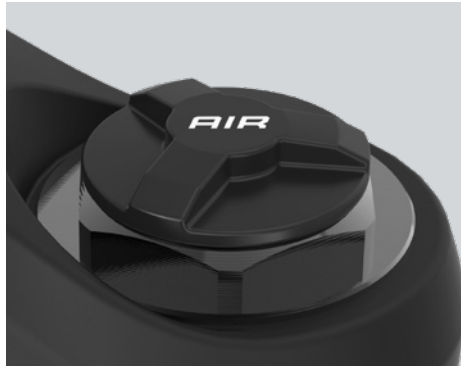
AIR EQ (3) Dual air spring system
