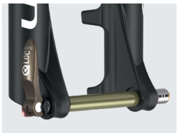
15QLC2 / 15QLC2-110 Ø15mm, O.L.D.: 100mm / 110mm Weight: 112g/115g
