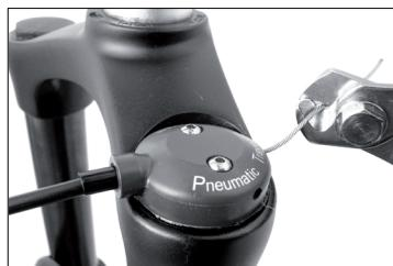
Install a cable end cap at the end of the cut cable using a needle nose plier
