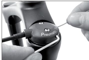
Cut the cable to a proper length. Approximately 12mm is recommended.
