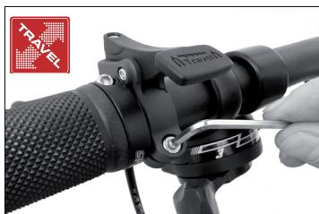
Thread the cable through the outer casing stopper and through the cable clamp. Tension the cable slightly and fasten it using a 2 mm Allen key
