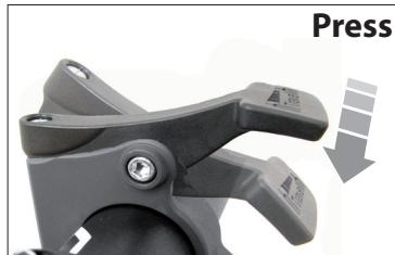
Press the Travel Adjust Lever downwards and hold it. Compress your fork. Release the lever again. Disburden your fork.
