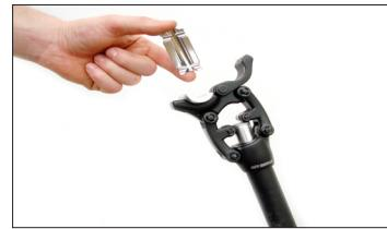
Place the upper clamp plate on to the saddle rail. Afterwards direct the gripper clamp through the two saddle rails and over the upper clamp plate.
