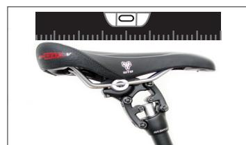
Fasten the two fixing bolts with 12Nm using a 5mm Allen key.
