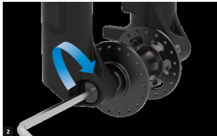
2 Tighten the axle with a 6mm Allen wrench by the suggested tightening torque of 8-10 Nm.
