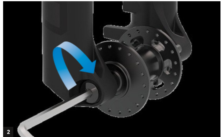
2 Tighten the axle with a 6mm Allen wrench by the suggested tightening torque of 8-10 Nm.
