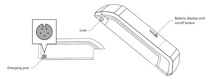
For safety this high energy density lithium ion battery contains a sophisticated battery management system (BMS). The BMS ensures safe charging and discharge, continuously monitoring each of the cells in the battery individually. If the current drawn gets too high or the temperature of the battery is elevated, the BMS will shut the battery down for safety.
