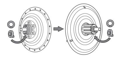
4. Tighten both wheel nuts to 40 Nm.
