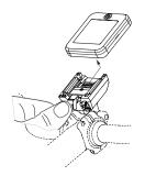
Slide up to cover the contacts and to prevent short circuits and malfunctions.
