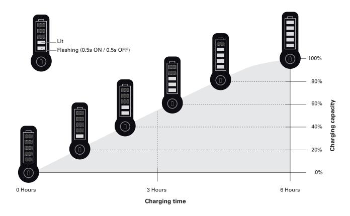
Every three months or after 40 sub-cycles, you should perform a complete discharge and recharge.
