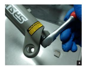
On the damper side, Install the washer and the black nut. Tighten to 8Nm and install the rebound knob (press).
