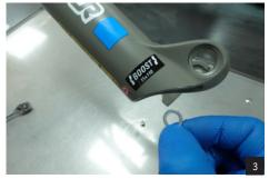
Use a long 10mm socket to unscrew and remove the nut and washer (Air side).
