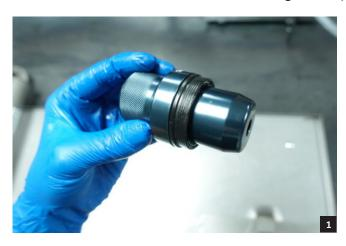
Hold the lower leg with one hand and finalize the installation tapping with a plastic mallet. Once you hear a change in the tapping sound, remove the tool and check that the seal edge is flush with the lower leg (picture 4). If necessary, repeat the process until the seal is flush with the lower leg.
