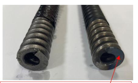
There are visible grinding and burn marks on both end of spring of fake product
