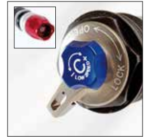
LO RC: Rebound adjust + Low speed Compression adjust + speed lock out
