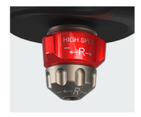
To open the low speed rebound: Turn the knob clockwise toward the (-) to open the low speed rebound. Result: The global rebound speed is faster.
