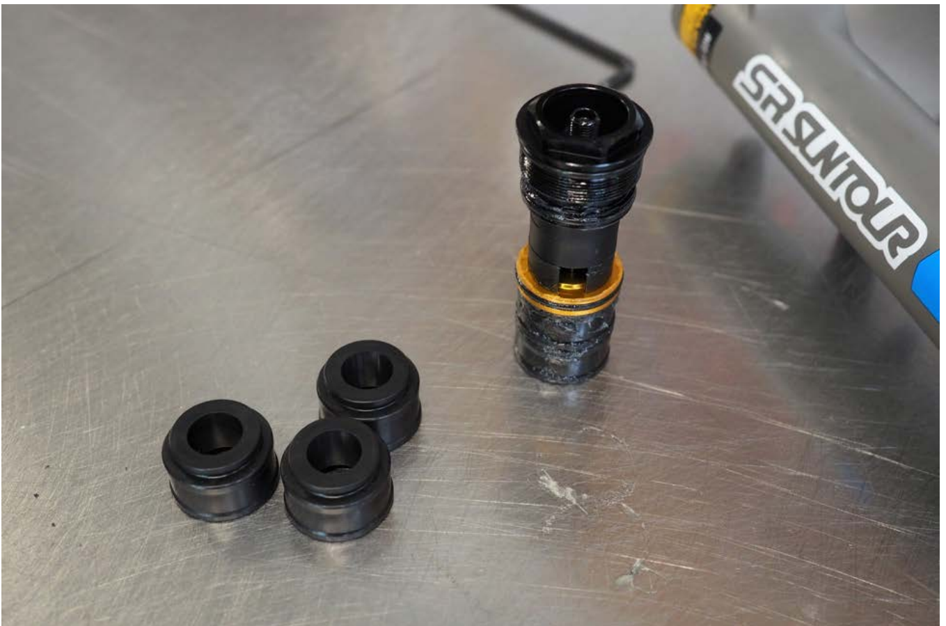
Just pull the airside top cap to change volume spacers. Rather than the older swap-system , they're now just rubber bumpers that are added or removed.
