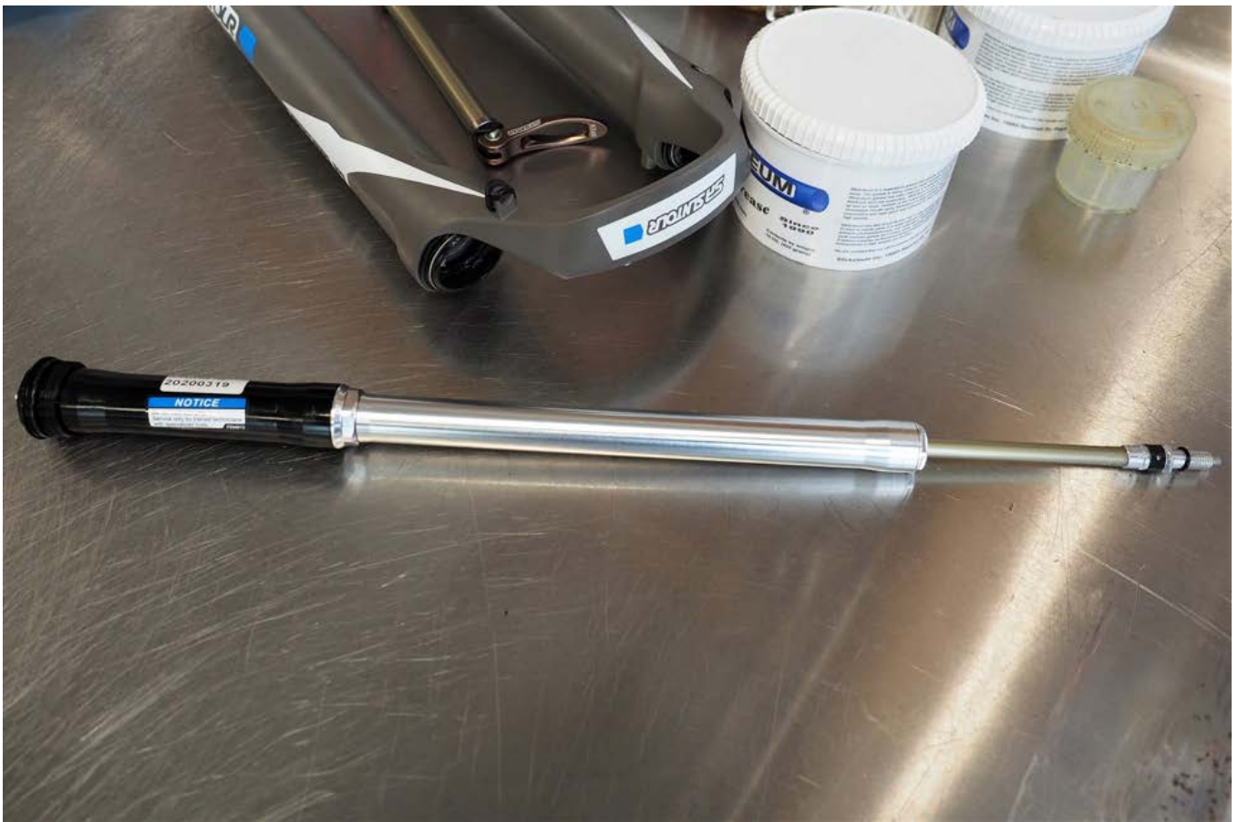
The familiar SR Suntour RC2 PCS damper. The newest generations of these dampers are much quieter than earlier editions.
